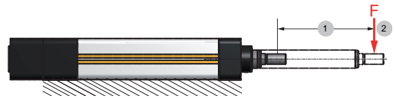
1: Extended length 2: Force application - at the middle of the cylinder rod thread
