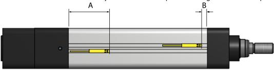
Figure 11: Position of sensors at the mechanical limits
