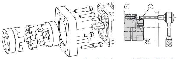
Figure 13: Motor/ gear assembly ETH100 ... ETH125 inline
