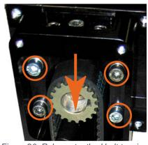
Figure 20: Release toothed belt tension
