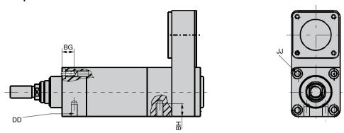
Figure 2: Motor parallel: ETH032 ... ETH080
