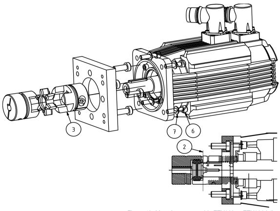
Figure 12: Motor/ gear assembly ETH032 ... ETH080 inline
