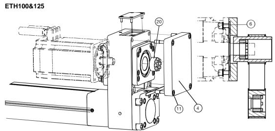
Figure 24: ETH1xx: Motor/ gear assembly parallel
