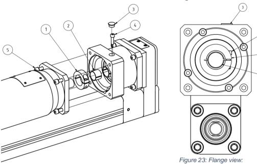
Figure 22: Disassembly of a EX motor
