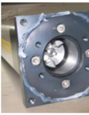
Figure 28: Flange prepared for IP65
