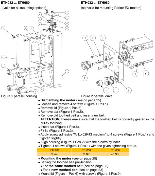
◆Mount lid (Figure 1 Pos.4) with screws (Figure 1 Pos.11).
