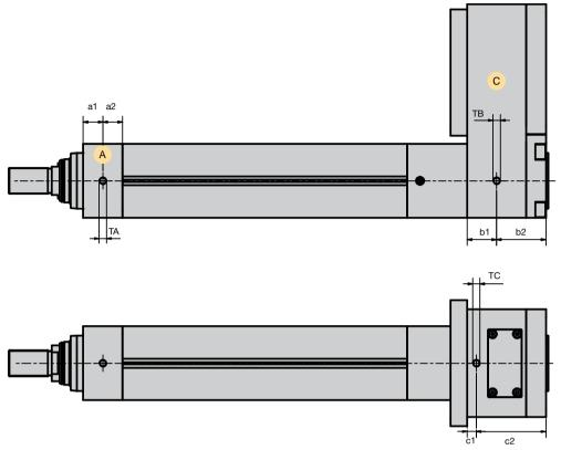
Figure 2 Transport instructions ETH100&125 Area A: Front cap Area C: Parallel housing Thread TA: on all four sides
