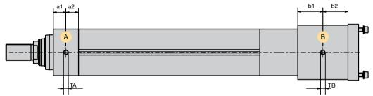
Figure 1 Transport instructions ETH100&125 Area A: Front cap Area B: Inline coupling housing Thread TA and TB: on all four sides
